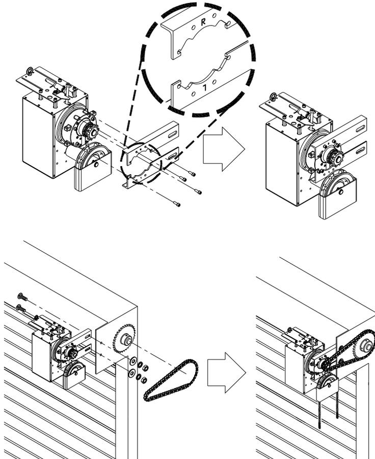
5. When the operator is mounted on the bracket, be sure the door sprocket is properly aligned / in the same plane with the operator drive sprocket before securing to the shaft.
