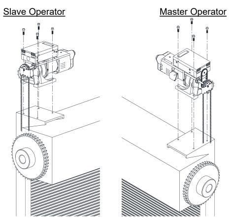
3. After mounting on operator at each side and before putting on the roller chain, checking the motor Rotation directions if both motors are correct through push the OPEN or CLOSE buttons.
