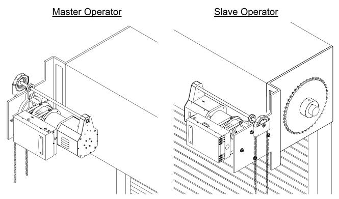
3. After mounting on operator at each side and before putting on the roller chain, checking the motor Rotation directions if both motors are correct through push the OPEN or CLOSE buttons.
