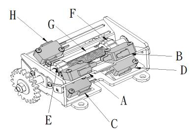
NOTE: "C" is usually the open limit switch and "D" is usually the close limit switch.
