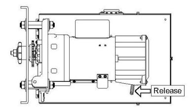
NOTE: A door sprung for emergency egress can open when the brake release lever is pressed.
