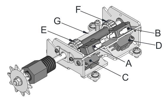
NOTE: "C" is usually the open limit switch and "D" is usually the close limit switch.
