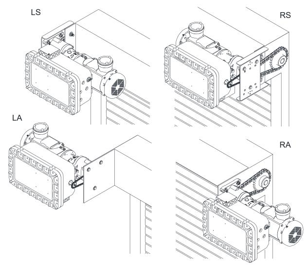
Installation positions for larger horsepower units are similar to as shown above.
