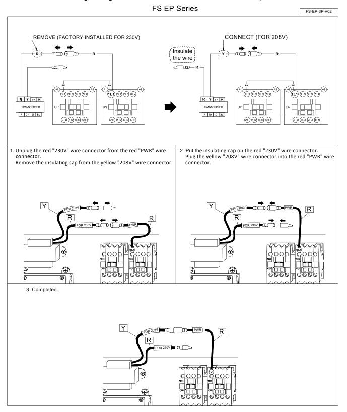
Wiring Change Instruction from 230V to 208V 3 Phase Operator
