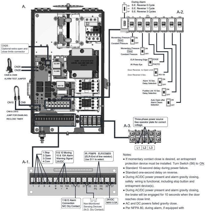
sensing device, door will stop on an obstruction after attempting to close the number of times selected on the S4 switch.
