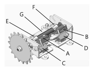
NOTE: "C" is usually the open limit switch and "D" is usually the close limit switch.
