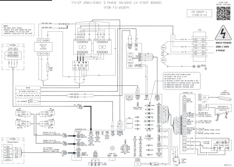
• REMOVE RED WIRE CONNECTOR AND THEN CONNECT TO YELLOW WIRE.
