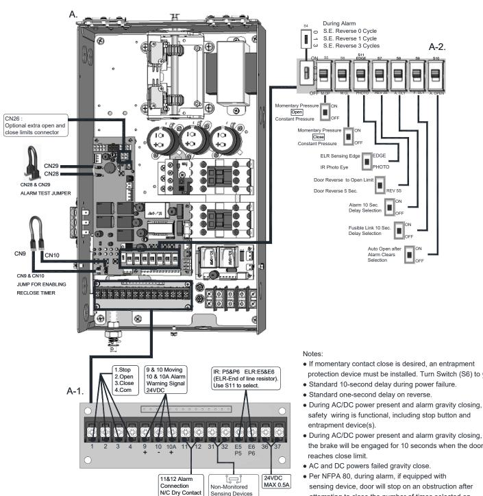
protection device must be installed. Turn Switch (S6) to ON.
