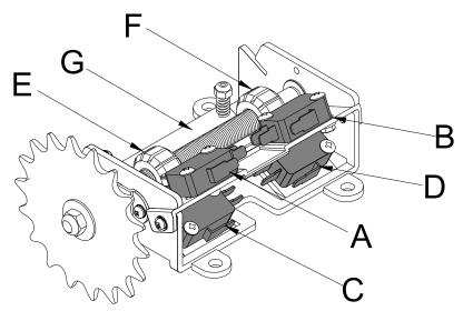
NOTE: "C" is usually the open limit switch and "D" is usually the close limit switch.
