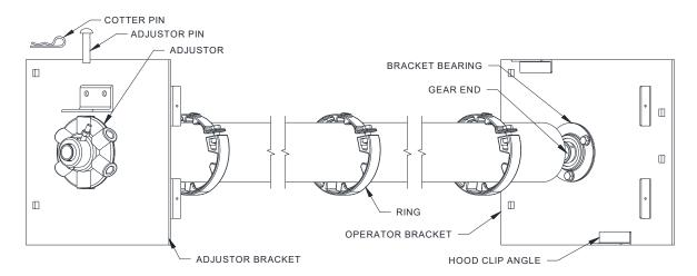
Figure 6.4 - Brackets and Barrel Prior to Installation
