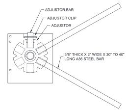
Figure 8.4 - SA0005 Spring Adjustor
