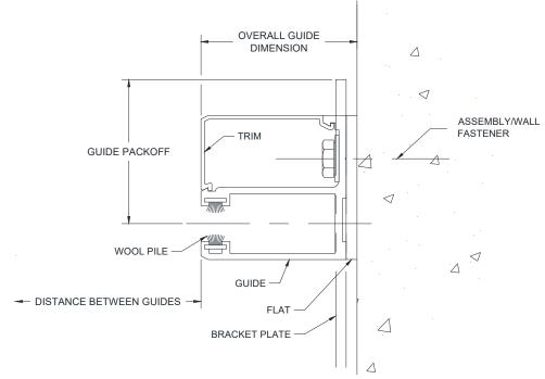
Figure 5.9 – Between Jambs with Back-Up Flat
