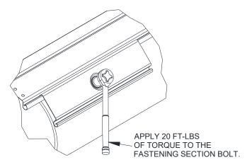
Figure 8.1 - Installing the Fastening Section
