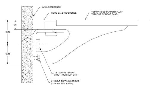
**Note:** See above detail for face of wall units; the wall angle is offset 5/8" from top of hood band to allow hood support to be flush while installing the hood.
