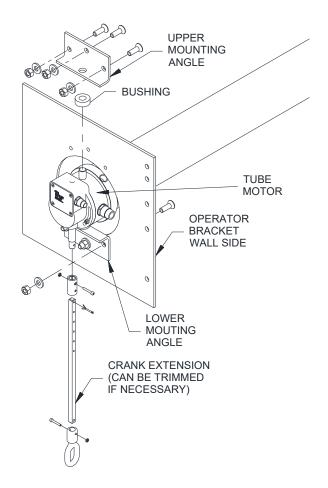
Figure 12.3 – 4" Shaft Assembly
