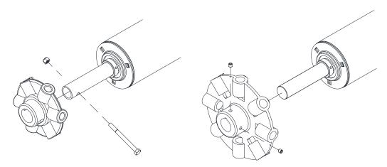
Figure 6.2 – Removal of Adjustor Wheel From Barrel Assembly
