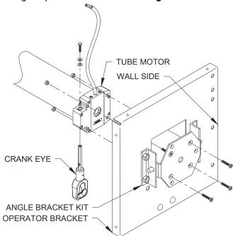
Figure 12.2 – 3" Shaft Assembly
