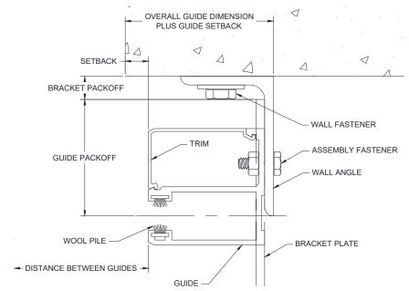
Figure 5.1 -Face of Wall "E" Guide
