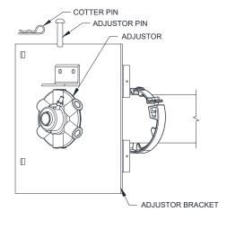
Figure 8.5 – Clamping the Guides, Applying Turns.
