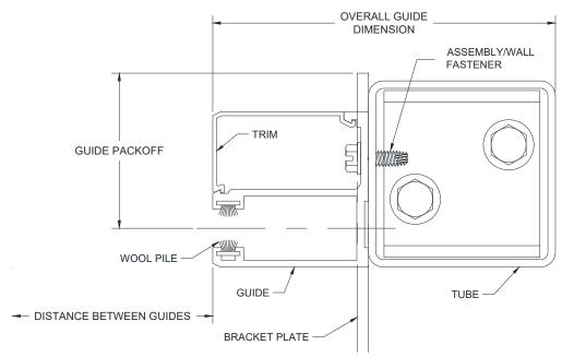
Figure 5.5 – Between Jambs Mounting to Free-Standing Tube
