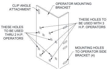
Figure 7.1 - Additional Operator Bracing
