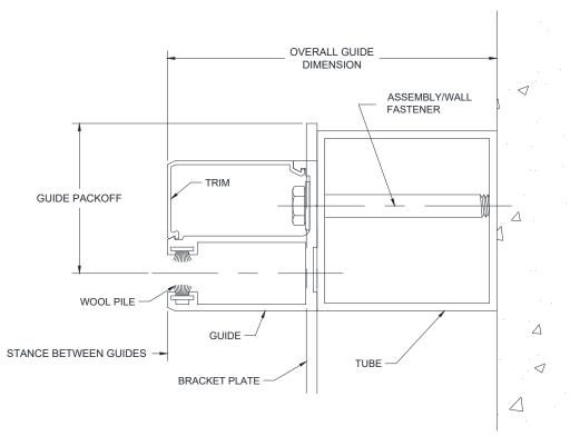
Figure 5.10 – Between Jambs with Tube Mounting to Wall
