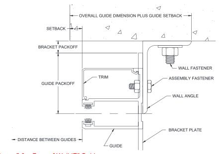
Figure 5.2 - Face of Wall "Z" Guide
