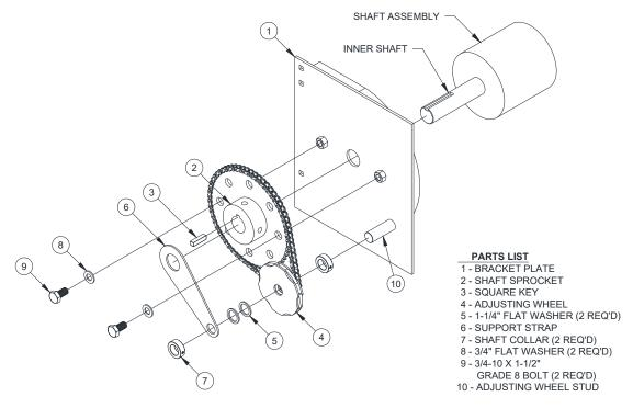
Figure 13.1 - Chain Sprocket Adjustor Assembly
