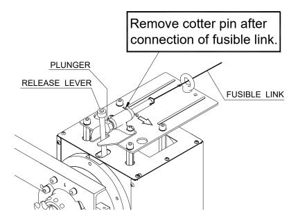
**NOTE:** Fusible link release can be substituted by an alarm release box. Fusible link release can be removed by loosening 4 screws. Alarm release can be attached by using the same 4 screws.
