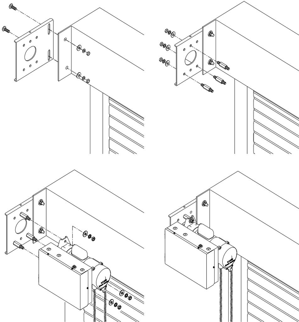
6. When the operator assembly is attached to the door bracket, be sure the door driven sprocket is properly aligned with the operator drive sprocket before securing the driven sprocket to the shaft.
