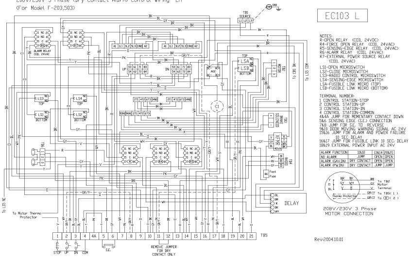
208V/230V 3 Phase (Dry Contact Alarm) Control Wiring LH
