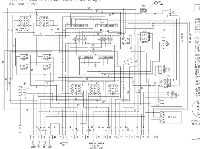
208/230V 1 Phase (Dry Contact Alarm) Control Wiring RH
