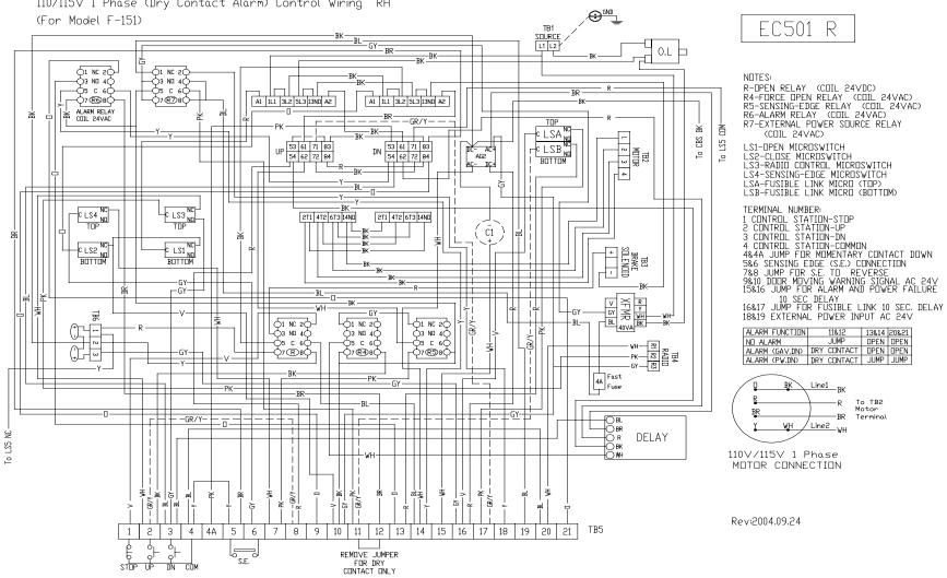
110/115V 1 Phase (Dry Contact Alarm) Control Wiring RH
