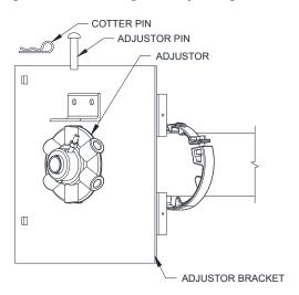
11. After cycling the door to the full OPEN and full CLOSED positions a minimum of 6 times, raise the door to the full OPEN position against the stops. If the door bottom bar is not level (within 1/4" across opening width), apply shims (Part No. 521870), as required, to adjust bottom bar level within 1/4".
