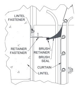
Figure 9.3 - "L" Shaped Lintel Seal
