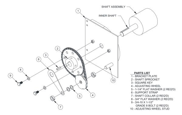
Figure A.1 – Chain Sprocket Adjustor Assembly
