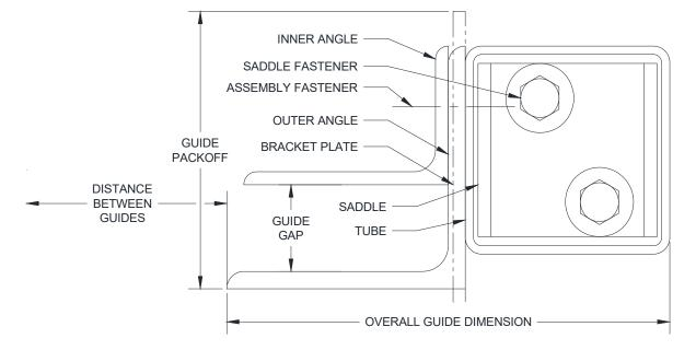
Figure 5.10 - Between Jambs Two-Angle Guide Mounting to Tubes
