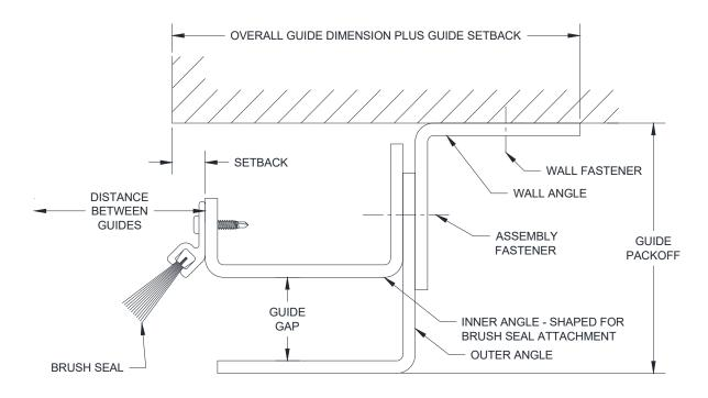
Figure 5.4 - Face of Wall "E" Guide
