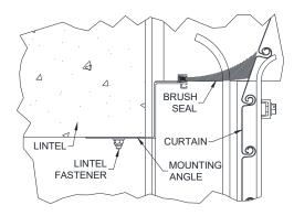
Figure 9.2 - "Z" Shaped Lintel Seal
