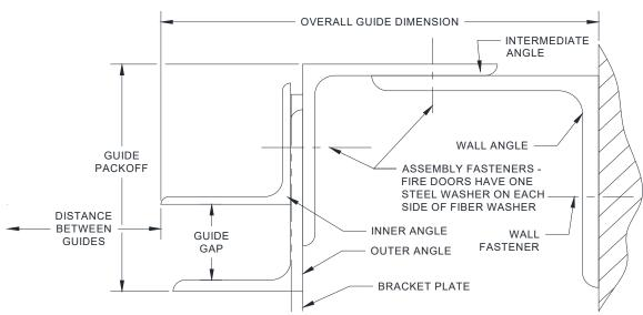
Figure 5.6 - Between Jambs Four-Angle Guide
