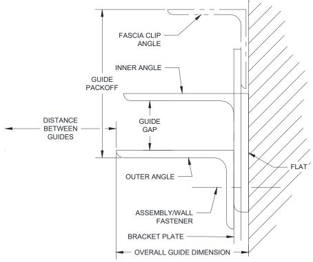
Figure 5.9 – Between Jambs Two-Angle Guide with Flat
