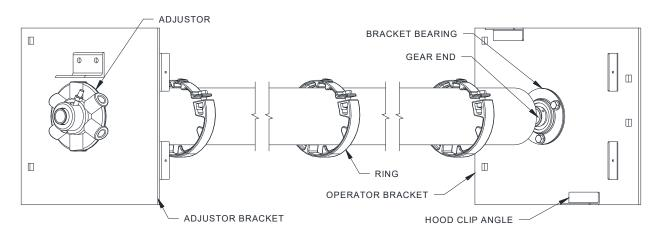
Figure 6.4 – Brackets and Barrel Prior to Installation
