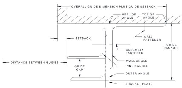
Figure 5.1 – Face of Wall "Z" Guide
