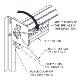
Figure 8.5 – Pinning the Adjusting Wheel
