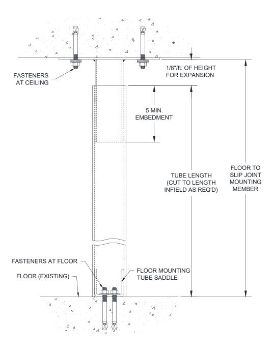
Figure 5.15 – Slip Joint - Floor to Wall with Plate Mounting Assembly
