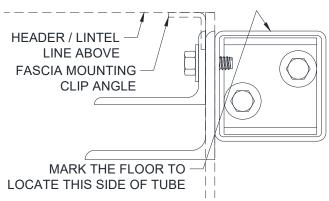
Figure 5.11 - Fascia Mounting Clip Angle
