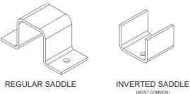
Figure 5.13 – Tube Saddle Hole location
