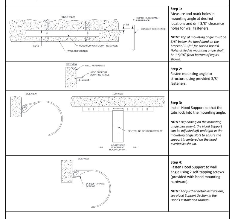
**NOTE:** Round Hood Support shown for reference, steps also apply for Square and Sloped Hood Supports.
