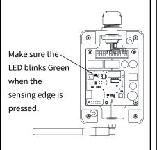
Step 8: Test the Sensing Edge Function with Door
