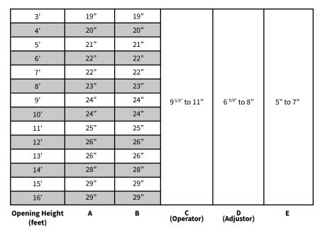
Maximum width between 13' 10" and 14' depending on configuration. Please contact the factory if maximum width required is more than 13' 10" to ensure proper configuration. Maximum opening width for CMU Mounting is 12'6".
