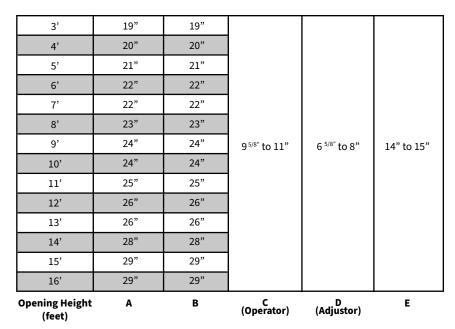
The maximum size available will vary slightly based on the wall construction. If the wall construction is steel, the maximum size is  $13' 11'_4$ " wide by 16' high. If the wall construction is concrete, the maximum size is  $13' 8^3/4$ " wide by 16' high.
