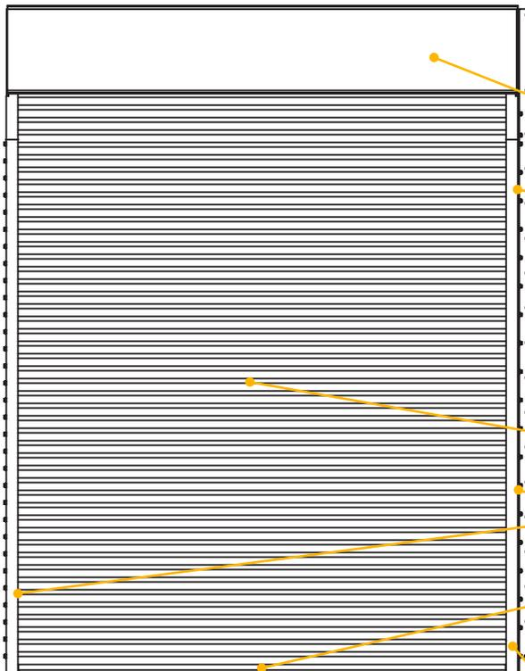
**BRACKETS** - Steel with powder coated finish to match curtain. Bolted to guide assembly and support counter-balance shaft and curtain.
