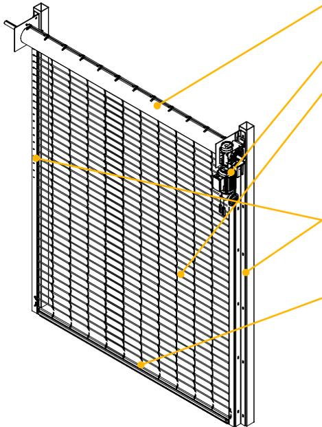
**SPRINGLESS SHAFT** - Steel pipe. Design reduces maintenance requirements and facilitate cycle capacity.
