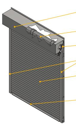
**HOOD** - Galvanized steel with GalvaNex<sup>™</sup> polyester enamel finish to match curtain. Encloses the curtain and provides fire protection at the head of the door.
