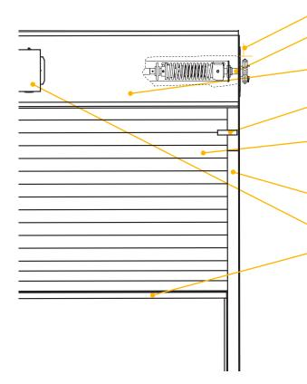
**BRACKETS** - 304 stainless steel with a zinc plated flange bearing.
