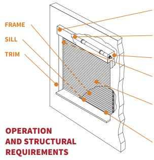
Chain hoist, crank and advanced motor operated selections allow you to further customize our product to fit your needs. Our coiling fire protectives are attached to the structural vertical jamb of the opening and supported by the guides. No additional support required unless hood supports are mandated by larger opening width.
