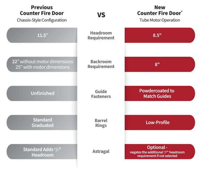
The new Counter Fire Door is available in manual push up and manual crank operation, as well as tube and chassis operators. FireGard (thermal activation) and AlarmGard (electrical activation) closing systems are also available on the new Counter Fire Door.
