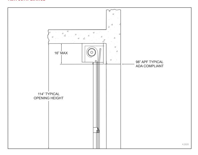
The Extreme High Performance MicroCoil Grille - 500K Cycles was designed with parking in mind. One of every six accessible parking spaces must be ADA van accessible in a parking garage. Since an ADA van only clears a typical opening of the parking structure by  $\sim 16$ ", installing a security grille used to be quite the challenge.
