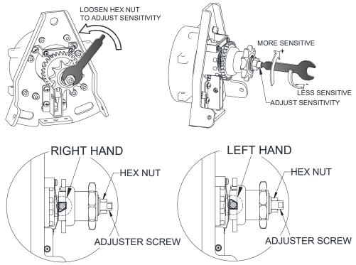
**<u>NOTE</u>**: 6 turns of the lock sensor adjustment will result in the lock sensor in the least possible sensitivity, which means the greatest amount of pull against the locking device. If the door is still not functioning properly, check spring tension, overall door installation and consult door manufacturer.
