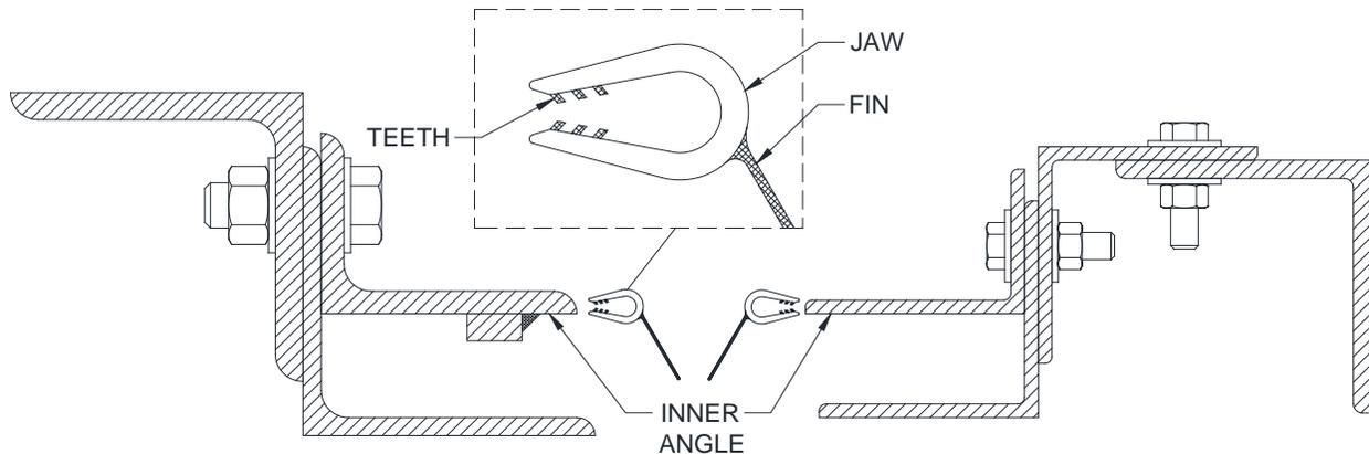
1. The seal should cover from the bottom of the bracket to the bottom of the guide. Check this by either measuring it or holding it up to the guide. If the seal does not cover from the ground to the bottom of the bracket, a spliced section is needed, proceed to step 2. If no splice is required proceed to step 3.
