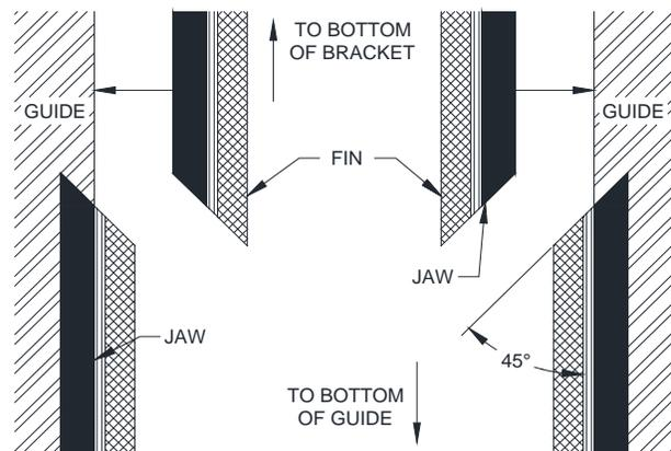
3. Start at the top of the guide and work downward. Be sure that the seal is fully seated on the angle.
