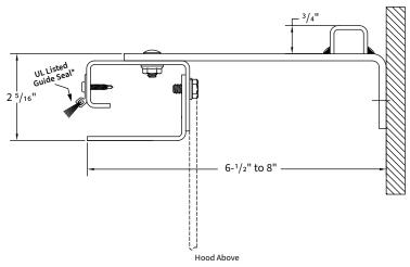
\*The UL listed guide seal is standard on model ERC11.
